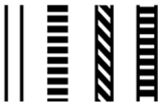
3S) A variety of crosswalk stripings are used in the United States. All are typically used in California except for the solid and the dashed. The standard would suffice for many intersections. Intersections with higher levels of pedestrian use, should utilize a spacing modified continental style (see 3S at the top of the page). Illustration credit: Dan Burden
