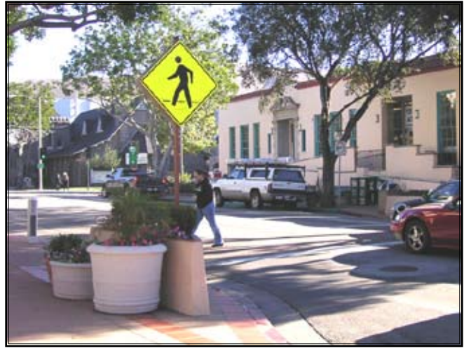
12S) This crossing utilizes lighting in the pavement and in the signs to indicate a pedestrian is in the walkway. Sensors pick up when a pedestrian approaches and if the crosswalk is clear of pedestrians. Photo credit: Mike Singleton
