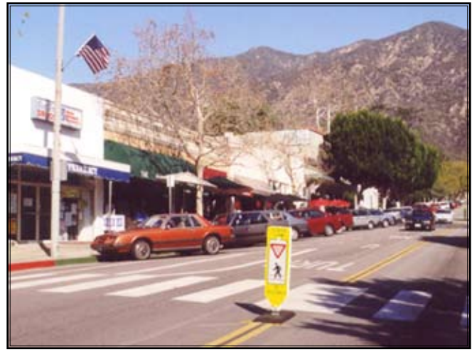
14S) If traffic control is not provided at an intersection, signage and striping along with a center pedestrian zone marker may help to make these crossings as safe as possible. This type of sign may require changes to existing San Diego policies, though it is allowed under MUTCD. Photo credit: ITE Pedestrian and Bicycle Council
