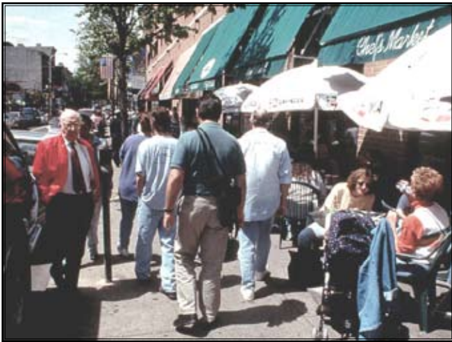
1W) Match the sidewalk width to the intended use. Only suburban residential areas should be allowed at or below a 5' width. Photo credit: Dan Burden
