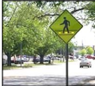
12S) This crossing utilizes lighting in the pavement and in the signs to indicate a pedestrian is in the walkway. Sensors pick up when a pedestrian approaches and if the crosswalk is clear of pedestrians. Photo credit: Mike Singleton
