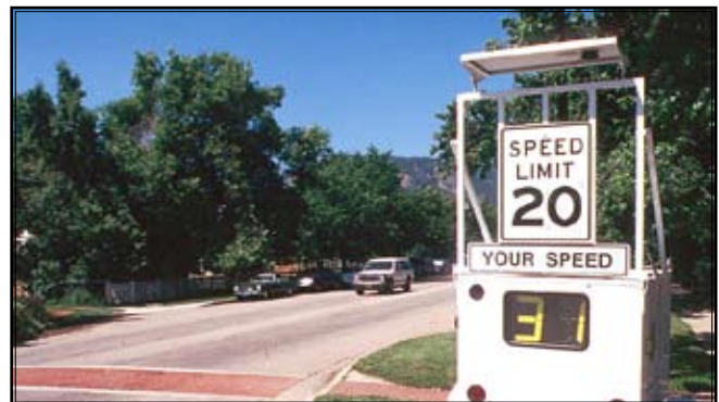
6S) Many cite increased regulation and enforcement as the solution to controlling speeding and reckless driving. Physical improvements provide a long term solution. However, some devices such as radar speed display systems, can help to educate the public and will slow the driver down while in use. Photo credit: Dan Burden
